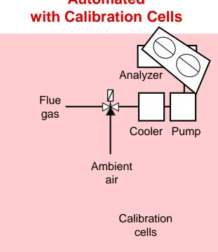
Calibration cells minimize operating costs and avoid the handling of test gases
